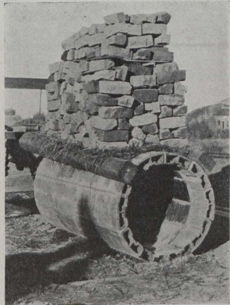
Fig. 2.—Test of Segmental Sewer Block Crushing Strength at Calgary City Yards.
