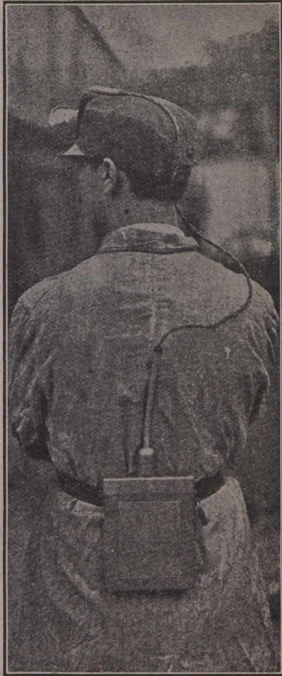
How the electric safety lamp is worn by a miner
