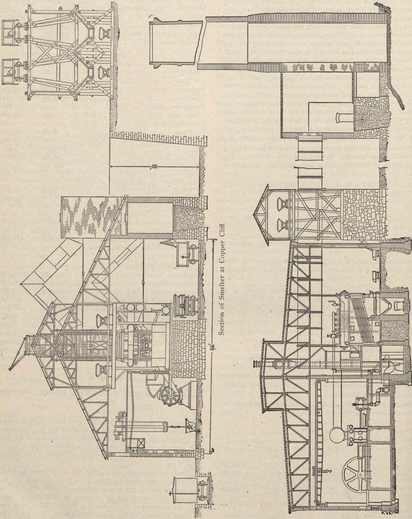
with the bins and also with the power-house, making a circular track, without switches, running on both sides of the furnaces and passing the coal chute in front of the power-house, which leads directly into the boiler room. The scheme of operation is as follows: Three miles from the plant is the largest mine. The ore is taken from this mine to the roasting-beds, which are about one-half mile from the smelter. After roasting, the ore is loaded into hopper-bottom cars
