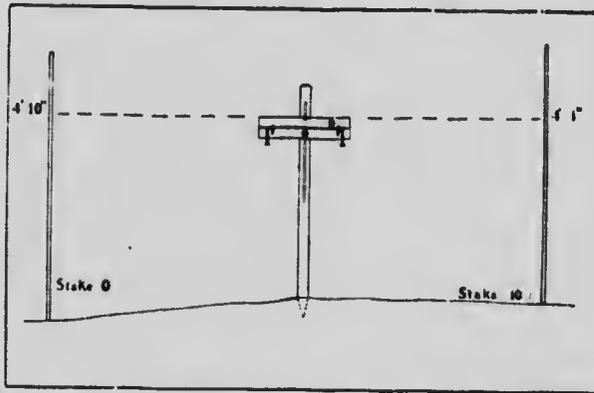
Fig. 2. Showing how to determine difference in elevation, using home-made drainage level.
