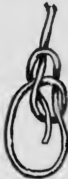
Bowline: a noose that neither jams nor slips.
