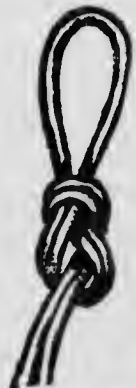
Fixed loop in middle of a cord.
