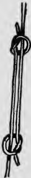
The fisherman's knot. It never slips; is easily opened by pulling the two short ends.
