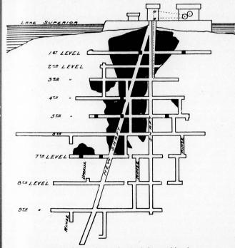
SILVER ISLET MINE—(part of the workings). Note :—Portion in black shows ore-body stoped. PE
