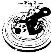
33111 Coté's Electric Circuit Switch.
