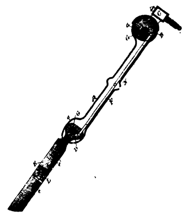
33130 Gunckel's Feed Water Regulator.
