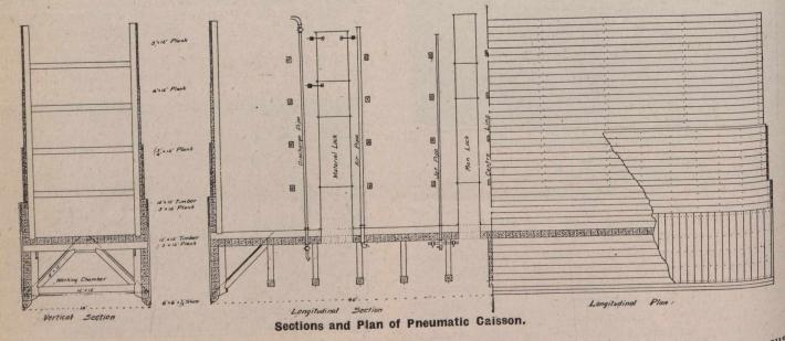
sure was used. The water inside the caisson being driven out under the shoe, the air men, or "sand hogs" as they are called, entered the caisson through the man-lock; and excavation began. Three eight-hour shifts of about twenty men each were worked continuously. The air pressure and upper
