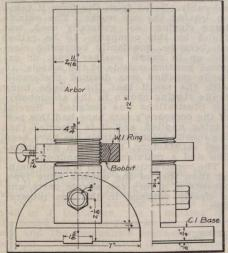
Jig for Carrying Commutator while Slotting in the Lathe.
