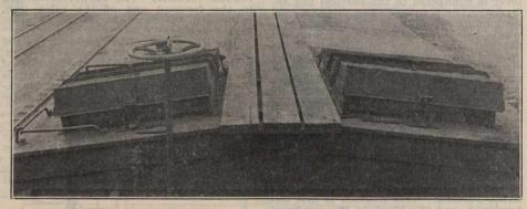
Fig. 3-Flap down to give Minimum Ventilation.
