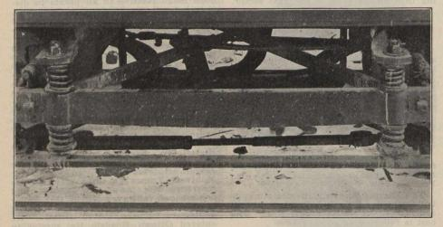
Inside Hung Brake Rigging on Hull Electric Co.'s Cars.
