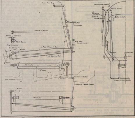
Fig. 1. Piping Arrangement on C.P.R. Oil Burning Locomotives.
