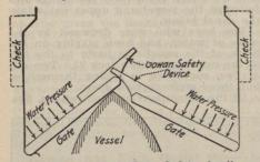
Fig. 5. Gowan Lock Gate Safety Appliance as fitted to a pair of Lock Gates.
