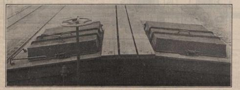
Fig. 4-Ventilator Closed and Clamped Down.
