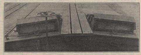
Fig. 2-Flap up to give Maximum Ventilation.
