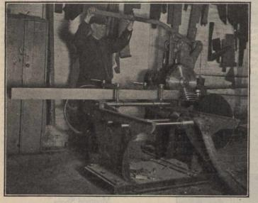
Fig. 2-Tie Plug Forming Machine Ready for First Cut.
