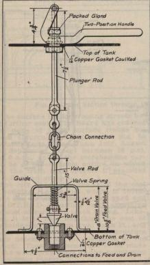
Fig. 2. Drawing Off and Drain Valves in the Oll Tank.
