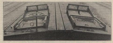
Fig. 1-Ventilator opened for Ice Filling.
