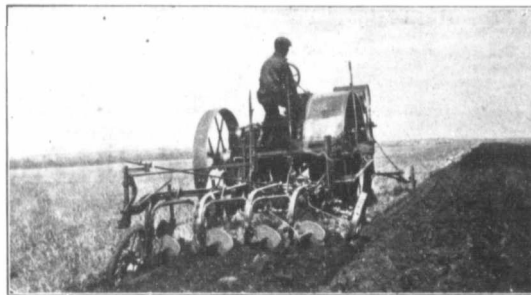
The motor is of the horizontally opposed type four cycle, two cylinder; 6 inch cylinder bore and 8 inch stroke. Fly-ball governor, high tension magnet, no batteries. It will burn gasoline, kerosene or distillate, and will develop a 12 horse power traction pull or 24 horse power on the belt.
