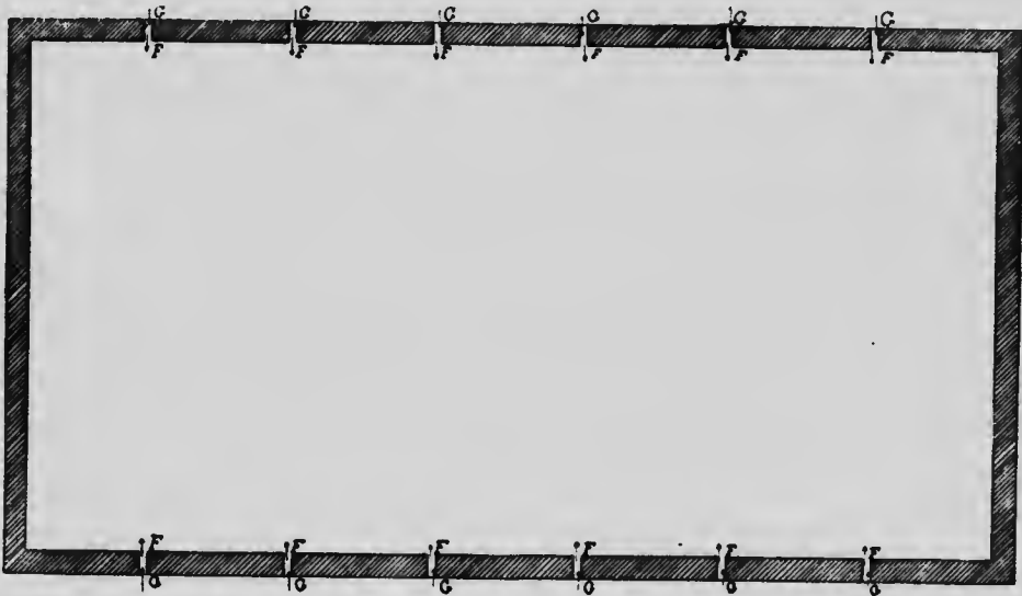
Fig. 5. Plan devised by Prof. King, of Wisconsin. Horizontal projection showing fresh air inlets.
