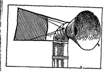
which should be made of galvanized iron, and arranged to revolve easily. Unless pretty sure that local shops can turn out first-class work of this character, it will be prudent to send to parties who are accustomed to doing such work.
