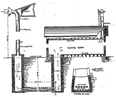
of the tile project. At the outer end erect an intake flue or pipe, which may be of wood or iron, and should reach well above any surrounding buildings or trees, (30 feet high in some places and 50 to 75 feet in others), and surmount it with a vane and cowl, so that it will catch every passing breeze, send it down the shaft, into the duct and thence up into the curing room and out through the ventilating pipe.
