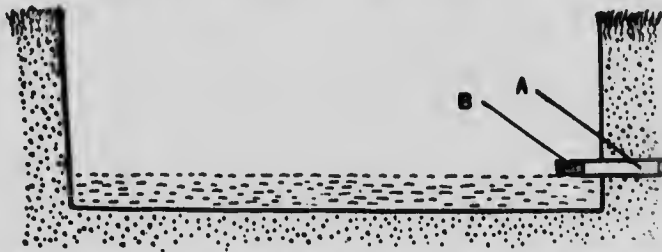
FIG. 9.—Tank ready for filling with flax. A. Outflow pipe. B. Wooden plug.
