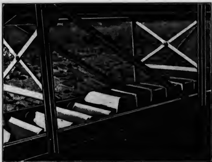
Dumping the wet peat bricks on the field: Royal Bavarian peat bog, Rosenheim, Munich.
