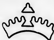
FIG. 45. Replacing Broken Tooth in Clock Wheel.
