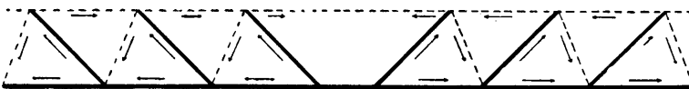
Diagram showing the action of the Kahn Trussed Bar, indicating the lines of stress. Note that the concrete takes all compressive stresses and the steel all tensile stresses. NOTE THE TRUSS ACTION OF THE BAR
