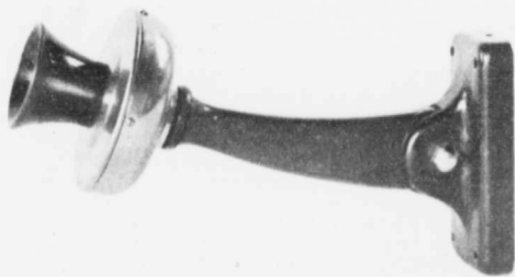
Fig. 73 Solid-back transmitter and transmitter arm
