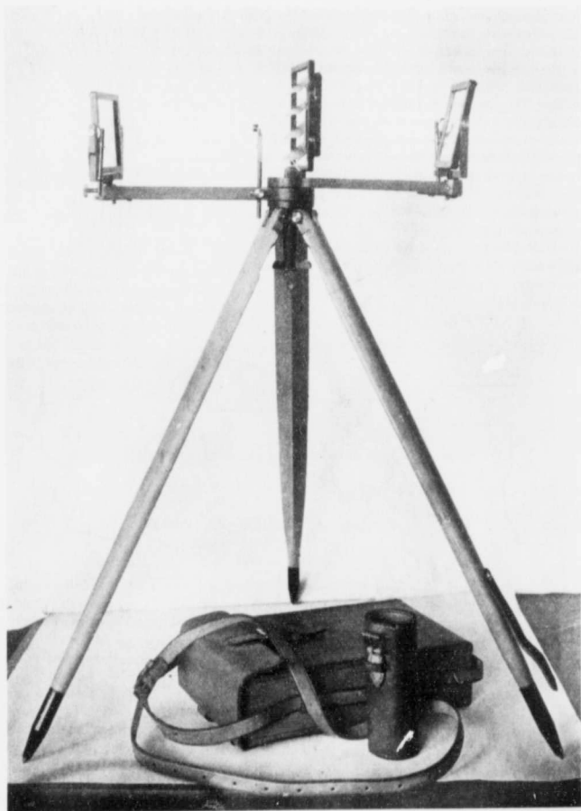
Fig. 103 Forest Service type of heliograph, two-mirror
