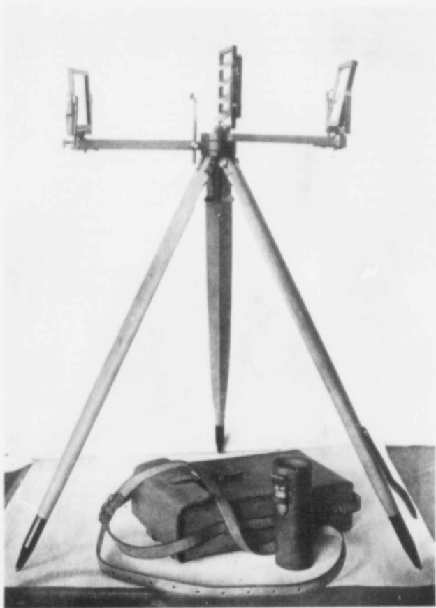
Fig. 103 Forest Service type of heliograph, two-mirror
