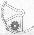
This is an external gear used on other mowers. Do you see the difference? These two wheels don't agree together so well. They have op-103 posite tendencies. The big wheel scratches and scrapes at the little one Sto and the little one tries 220S hard to get away from the big one.
