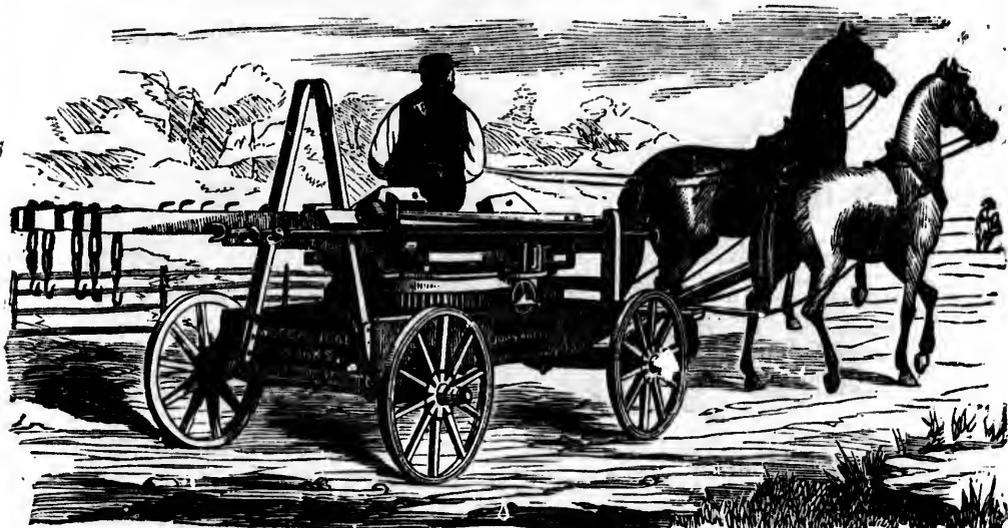
MOUNTED TRIPLE GEAR POWER AS LOADED FOR TRAVELLING.
