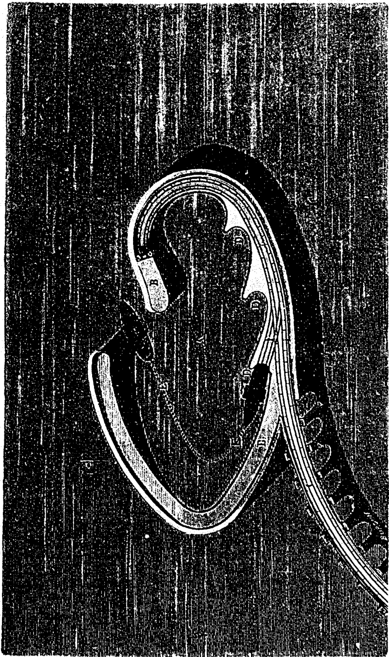
THE HARBOR AND DYKE PROJECTED BY M. DUPUY DE LOME. A. Basin. B. Dyke. C. Railway and Bridge. D. D. D. Shipping wharves. E. E. Outward bound channel. F. Drawbridge regulated by the height of the tide.
