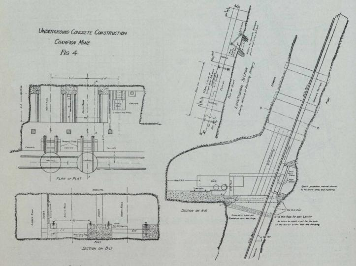
Sections and plan showing underground concrete construction, Champion mine
