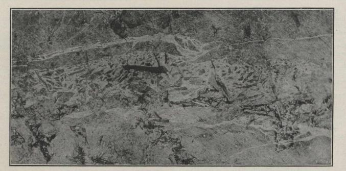
No. 1. vein, Tough-Oakes Mine. Gold quartz in brecciated porphyry
