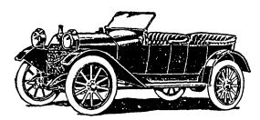
All modern improvements. Selective sliding gears—three forward, one reverse. Long-stroke motor. Gasoline tank in front of dash.
