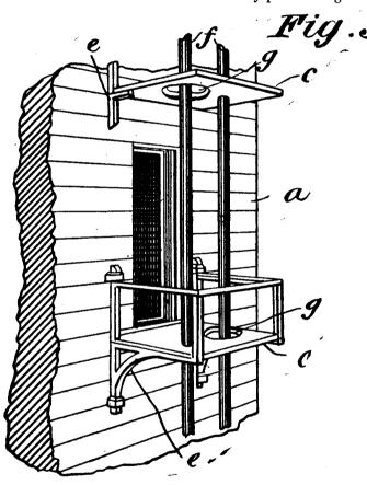
floors or staging from the root to the ground; g g are c cular openings which alternate from one side to the other at each succeeding landing. The landing to be placed before a window at every story.
