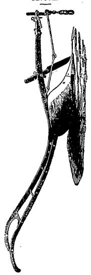
This cut represents a very strong, simple, and effective plough, manufactured by Ransomes & Sims, of England, an extensive and old established firm, of world-renowned reputation. It is specially adapted for breaking up ground recently cleared for cultivation, where a strong, rough, and ready implement is necessary. It has been
