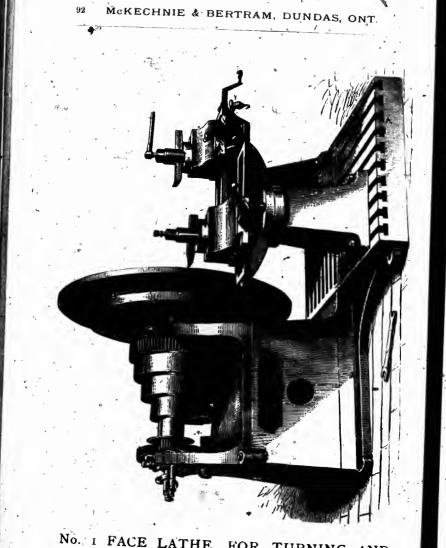
No. 1 FACE LATHE, FOR TURNING AND BORING PULLEYS.
