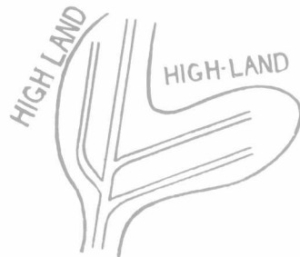
Fig. 4.—Drains adapted to suit the land.
