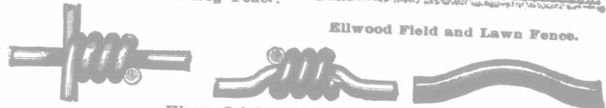
Hinge Joints and Tension Curves.
