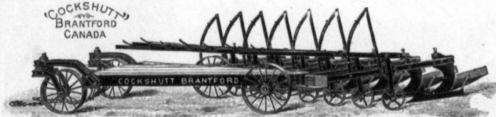
Seven Furrow Engine Gang. Equipped with breaker bottoms, fin cutters and extra shares, or stubble bottoms and swivel rolling colters. Also made in 6, 8, 10 or 12 furrow sizes.
