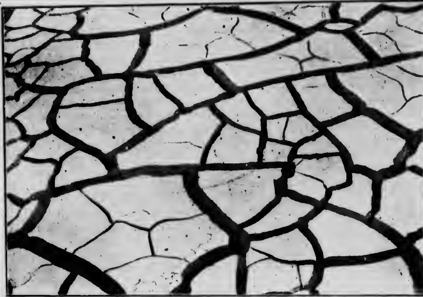
Fig. 70.—Strong clay left by potter to dry. Note shrinkage of clay on drying; hence necessity for adding sand to strong clay in brick-making to prevent cracking when drying.
