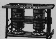
Burns with a clear blue flame, without smoke, and a heat of the greatest intensity. Burners are brass, and so made that wicks can be replaced in a few minutes as in an ordinary lamp. Wicks are 10 inches in circumference and should last one year.
