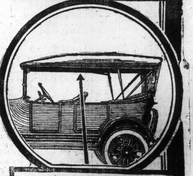
Perfect-fitting, "one-man" mohair top; quick adjustable storm curtains, rolled up inside of top.
