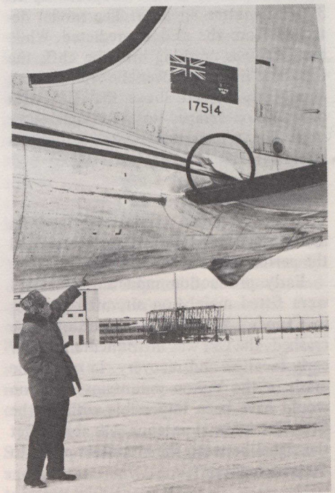
Harry Stevinson points to a CPI attached to a Canadian Forces' plane. The leading edge, held by a spring-loaded latch, is forced up when released, allowing the on-rushing air to lift the CPI away from the plane. High-speed planes are equipped with flush mounted CPI's.
