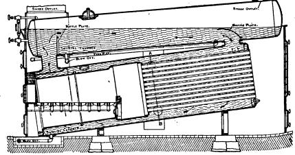
Has forced water circulation similar to a Water Tube Boiler, large effective heating surface and special arrangements for preventing and removing scale.
