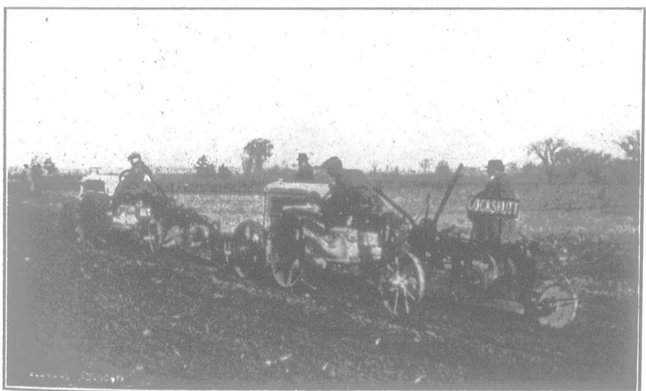
The Ford Tractor. One machine burning kerosene the other gasoline.
