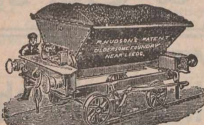
50—R. H.'s Patent 5-Ton Steel Double Side Tip Wagon, to work with ordinary Rly Wagons
