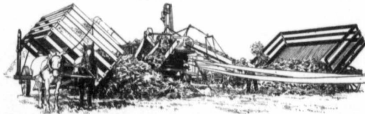
The above represents what is known as the Nelson Dump Rack. This rack is constructed in such a way that one side of the rack is raised by means of a windlass, thus discharging the load.
