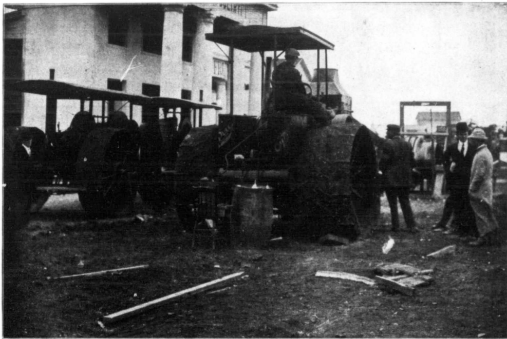
Rumely Oil Pull "E"—Holder of the World's Record on Fuel Economy Developing 67.99 Horse-Power in its Matchless Run on the Brake
