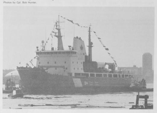
The vessel has a beam of 19.7 m and draws 7.2 m.
