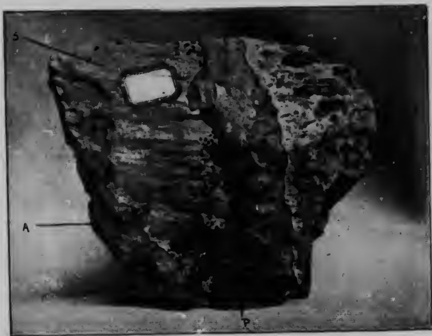
Specimen showing intimate association of apatite (A), scapolite (S), feldspathic rock (F), pyroxene (P), from the Star Hill mine, township of Portland West, Que.
