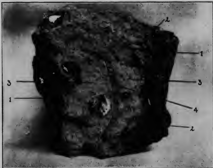
Piece of mica-apatite vein, showing mica crystals along the walls (1); next, a narrow zone of small, spangle mica (2); vein filling of granular "sugar" phosphate (3) with included mica crystals, and, in the centre a narrow strip of pink calcite (4). In the original specimen there is a close approach to development of flow structure, which is lost in the photograph; this structure is probably due to incipient parallel banding of the mica and phosphate particles, caused by squeezing of the vein. Specimen from range I, lot 16, township of Wakefield, Que.
