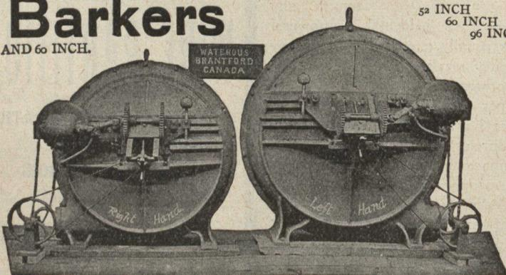
Heavy machines, thoroughly well made, for fast continuous service—made either hand, down or up delivery. WITH OUR cutting up rig 2 men handle 100 to 125 cords per day, taking logs from water, delivering cut wood to barkers in any length. Special cross cut machines also supplied for handling shorter or smaller wood.
