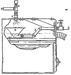
A - Represens Air Vessel on feed wate pipe, made of 1 to 3 in, iron pipe and 2 to 4 ft. hlgh, according to space available.
