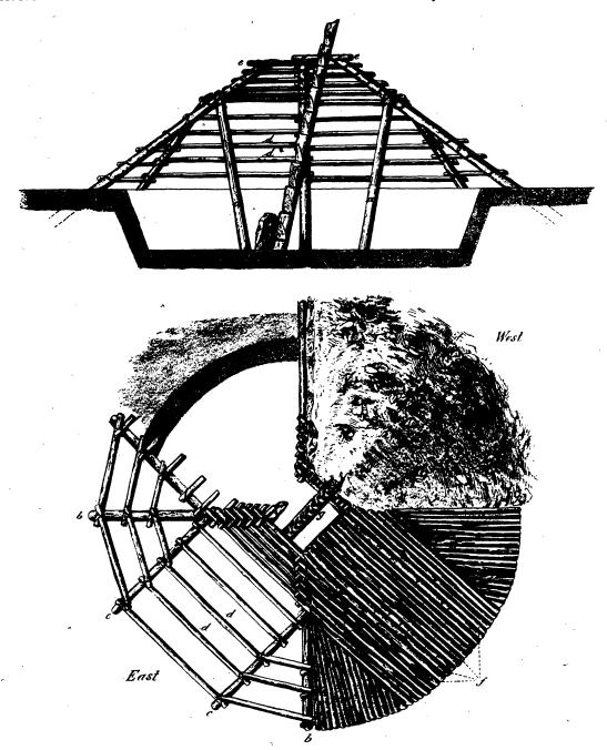
Figs. 135, 136. Plan and Elevation of Underground House.
