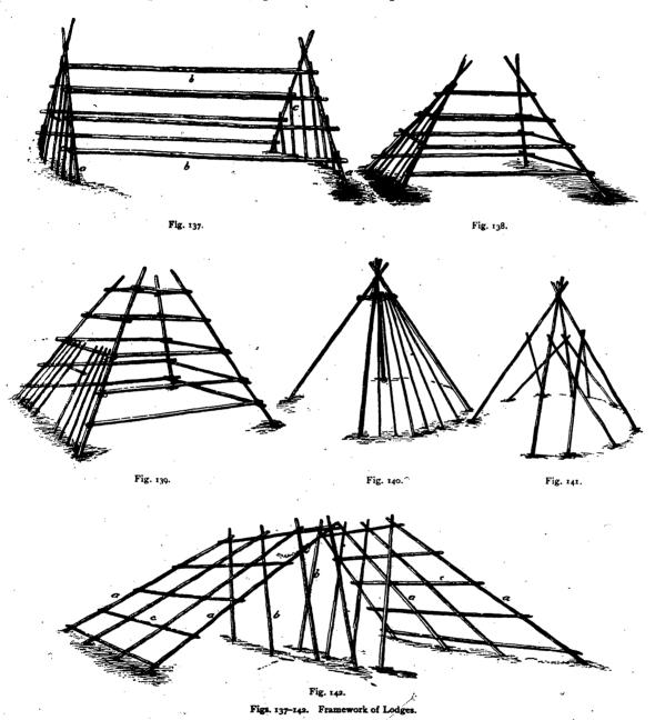
the bark out. The Lower Thompsons use cedar-bark only. Frequently the temporary lodges of the Lower Thompsons were only a single slanting roof, similar in construction to the large shelter described before (Fig. 142), but much smaller.
