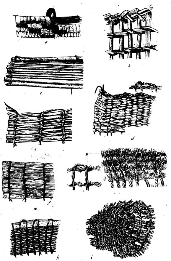
FIG. 131. DETAILS OF WEAVING.
