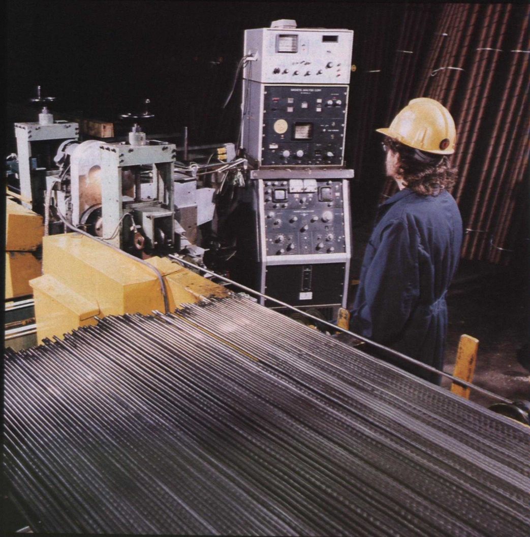
▲ Checking for tight seams and surface defects not readily visible using a Roto Bar non-destructive testing unit
