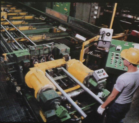
▲ Checking for tight seams and surface defects not readily visible using a Roto Bar non-destructive testing unit
