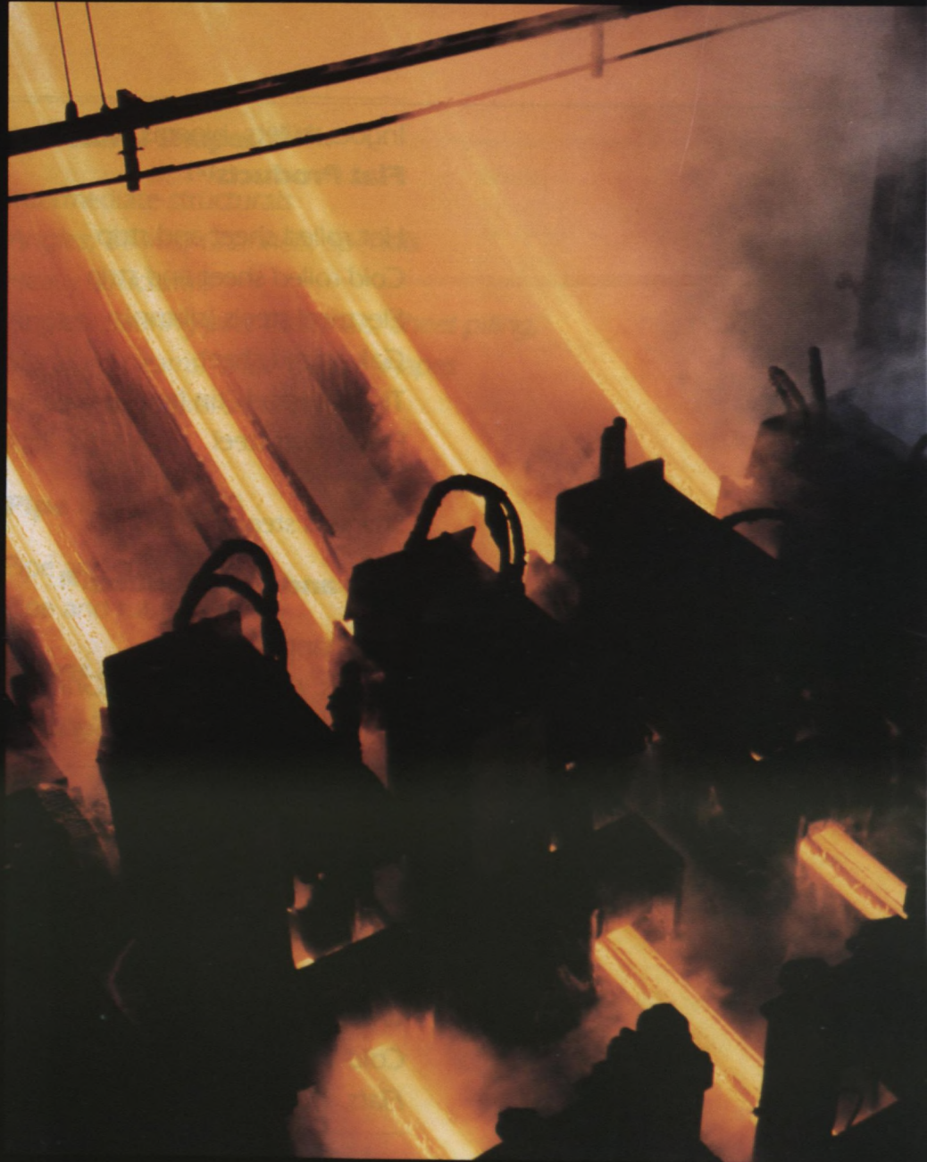
▲ The Rokop four strand continuous casting machine.
