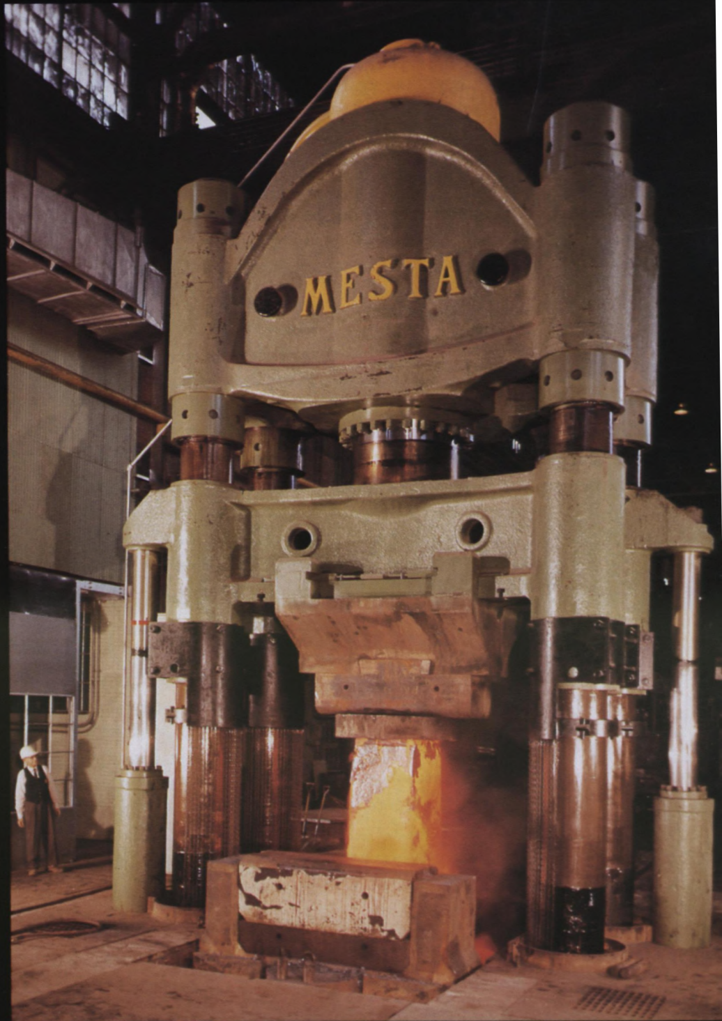
▲ The 5 000-ton [4 500 tonne] forging press at Sorel
