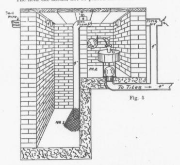
low the surface, and must be perfectly level, for the reason that if given a fall the earth surrounding the low edges of the system would receive more than its share of liquid sewage, and might in time become fouled, while if level, the earth surrounding every tile has an equal amount of work to do, and will produce most satisfactory results.
