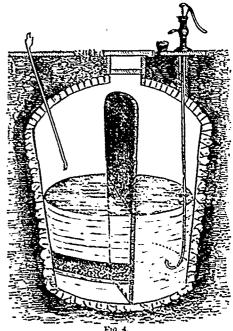
We give below, in round numbers, an estimate of the capacities of cisterns of various dimensions. A cistern five feet in diameter will hold a little over five barrels to each foot of depth.
