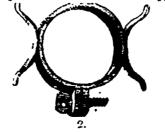
a wooden handle cut out in the centre like a clothespin, (fig. 1). A whole stone or a broken half of one, is securely fastened by turning the screw, which eaables one to use up fragments, or to use very short stones; while the flanges guard the hand from being cut, if a wrong movement happens to be made. American Agriculturist.
