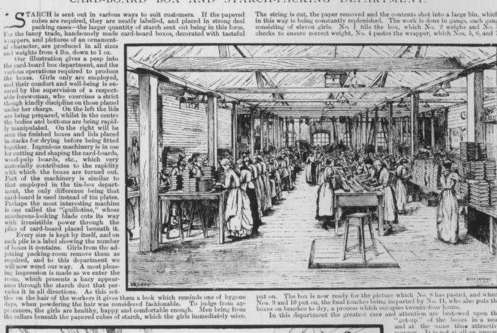
put on. The box is now ready for the picture which No. 8 has pasted, and which Nos. 9 and 10 put on, the final touches being imparted by No. 11, who also puts the boxes on benches to dry, a process which occupies twenty-four hours.
