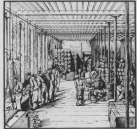
To prevent the delicate colour work being damaged by friction during transit, the tin is then wrapped in paper and put on oneside until required by the packers.
