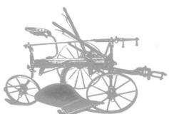
When you buy a NEW ECLIPSE PLOW, you get full value because Frames and Beams are of high carbon steel and guaranteed not to break or bend.
