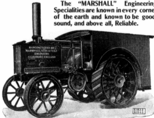
The above represents a 32 H.P. Draw Bar and 60-70 Brake H.P. "CLASS F" Tractor, with two travelling speeds.
