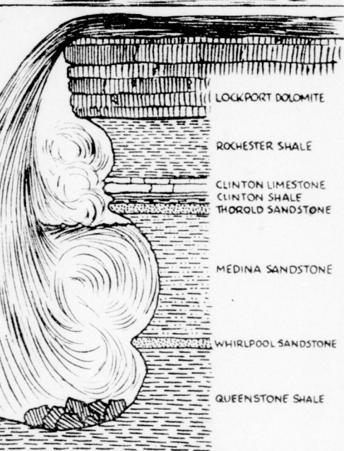
THE RIVER DOES NOT TEAR BLOCKS OUT OF THE ROCK ABOVE BUT UNDERMINES THE CLIFF INSTEAD. A TYPICAL CROSS-SECTION OF THE HORSESHOE FALLS.
