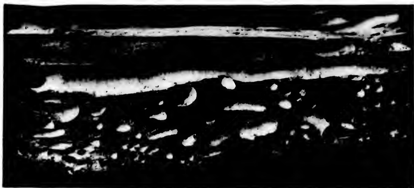
FIG. 14.—Spruce submerged two years in Coal Mining Company's wharf, Middle River, Pictou, N. S. four feet below low water.
