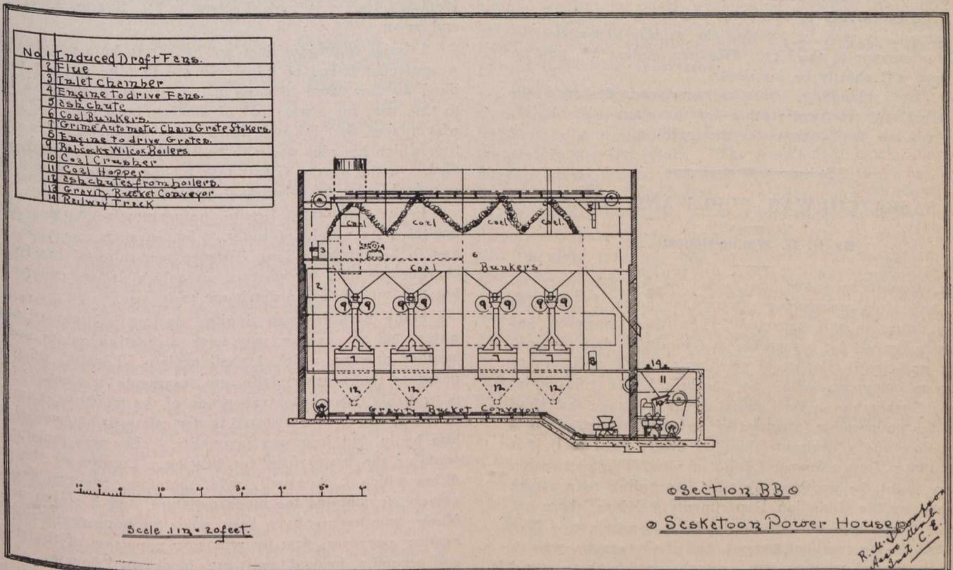
extend down to the hoppers of the stokers, and a steady flow of coal from above supplies the stokers at all times. The overhead bunkers are kept filled by a gravity bucket con-
