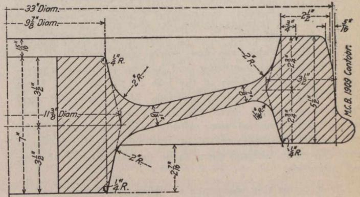
Fig. 2.—Steel Wheel for Tenders, Freight and Passenger Cars.
