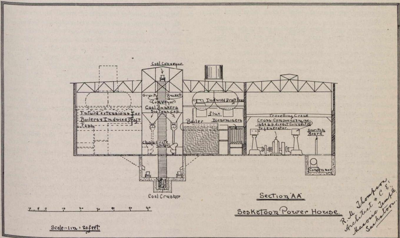
tion of a set of steel coal and ash bunkers, which extend the full width of the building, and are placed immediately above the boiler fronts and stokers. From these bunkers chutes
