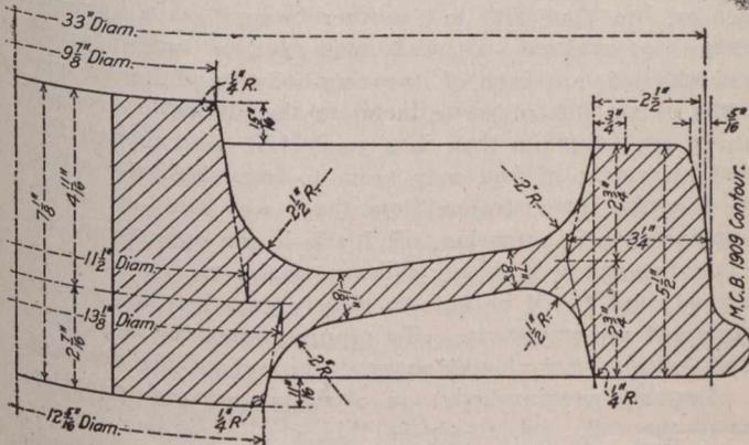
Fig. 1.—Typical Design of Solid Steel Engine Truck Wheel.
