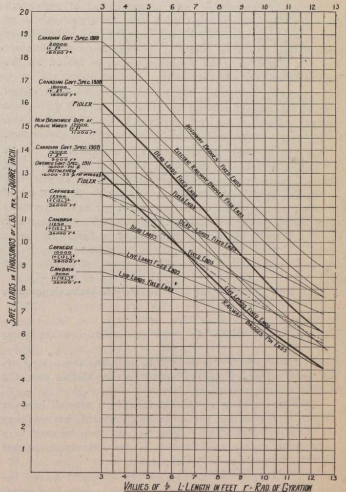
The other two curves belonging to the same specification—one for electric railway bridges and the other for railway bridges—would be reduced in a similar manner, but have not been shown.
